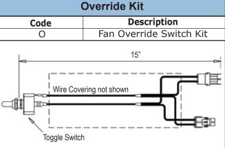
The Override Kit includes a toggle switch which allows fan activation. Use this option in conjunction with one of the Switching Kits (ASW, GSW, TSW).
