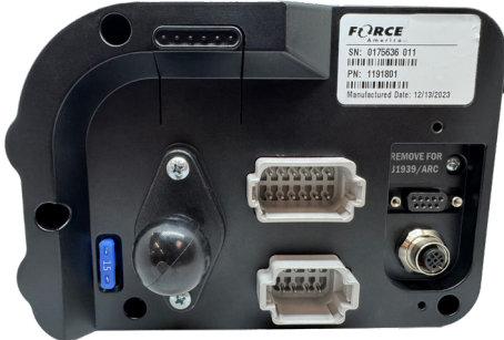
Tactically placed interlock button to ensure safe use of critical functions.
