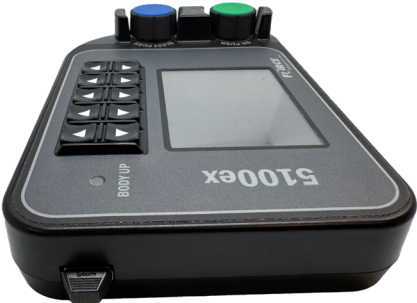
Built in USB port for data retrieval and firmware upgrades.
