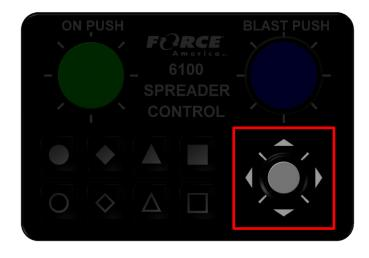
The touch screen navigation controls area and Nav Stick joystick provides a way to change between views on the screen, select panes of Soft Switches, and make adjustments to settings. The up, down, left, right, and select functions can be done using Nav Stick on the operator interface or also with the touchscreen on the display.
