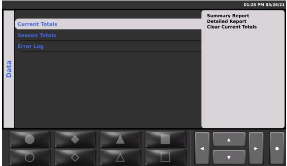
The Data Menu allows you to view, export, and clear data totals and error logs collected during the SSC6100 system's operation.
