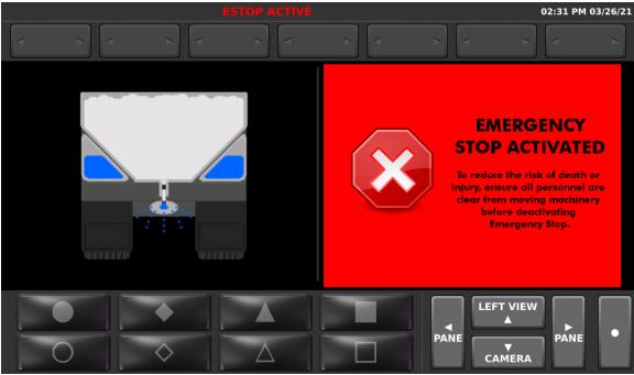
The SSC6100 has an emergency stop feature that is activated by pressing the red ESTOP pushbutton located near the Operator Interface control. When ESTOP is activated the screen shows the red Emergency Stop Activated message and a buzzer sounds. In addition, all outputs are immediately shut off, the system enters Standby mode, and if the system is configured with a Low Oil PTO or diverter valve, these will be shut off as well.
