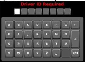
For the Numeric or Alphanumeric Driver ID modes, enter your numeric Driver ID using the onscreen keypad and press the Enter button.
