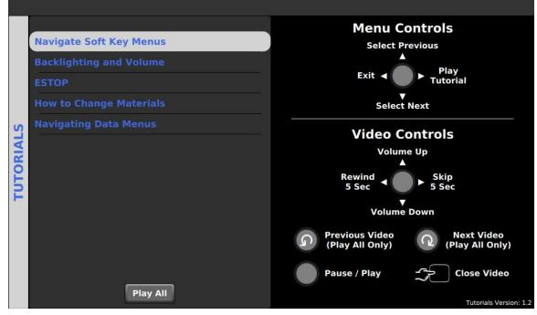
The Tutorials Menu allows you to watch various tutorials on how the spreader control operates. To access the Tutorials Menu, scroll to the MENU Soft Switch pane and press the Tutorials Soft Switch.
