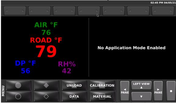
For systems equipped with a PreCise®MRM ARC sensor, pressing the Navigational Control "LEFT VIEW" up direction can bring up a view that shows the current Road Temperature, Air Temperature, Dew Point and Relative Humidity.
