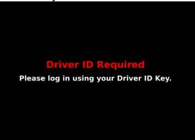
This method requires a USB driver key to log in to the system. Insert a pre-programmed USB Driver ID Key into either of the USB ports on the lower right side of the screen. Additional driver ID keys can be programmed in the Calibration menu. See the SSC6100 Calibration manual for more information.
