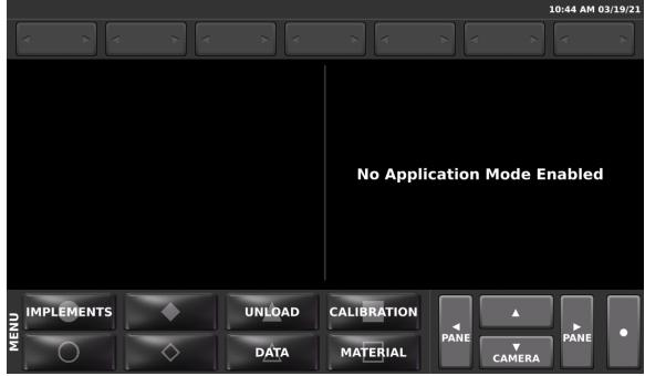
Selecting an Implement type of "None" is generally used to disable seasonal functions and prevent accidental activation of hydraulic functions. In this mode, the spreader functions will not run, but Joystick functions will still operate normally.
