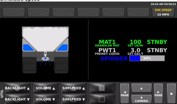
If enabled, the SSC6100 can simulate a ground speed signal instead of using the actual speed signal from the vehicle. When activated, the simulated speed overrides the vehicle speed unless the actual vehicle speed exceeds 5 MPH.
