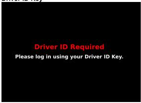
This method requires a USB driver key to log in to the system. Insert a pre-programmed USB Driver ID Key into either of the USB ports on the lower right side of the screen. Additional driver ID keys can be programmed in the Calibration menu. See the SSC6100 Calibration manual for more information.
