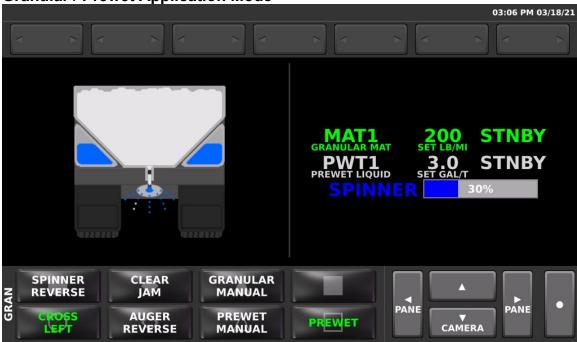
This mode applies granular material with the option to apply prewet.
