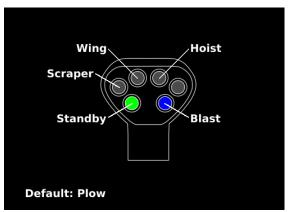
The specific functions of each joystick systems are custom configured at the factory for each vehicle application. An on-screen guide of these functions can be brought up by pressing the Navigational Control "LEFT VIEW" or joystick Up direction until the joystick guide is displayed.
