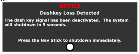
The 6100 automatically begins a shutdown process when power is no longer detected from the key switch. A built-in timer prevents the system from shutting down during engine starting.
