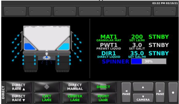
Simultaneous Granular / Direct application mode allows both the granular / prewet system and the direct liquid system to operate at the same time.
