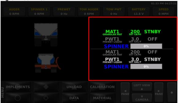
The right window by default displays spreader rate information. If enabled, this window can also display camera images. Pressing down on the Nav Stick Pushbutton, or the down arrow on the Nav Stick will cycle through camera images, if equipped. If the spreader power switch is off, the spreader screen with display "Spreader Off".
