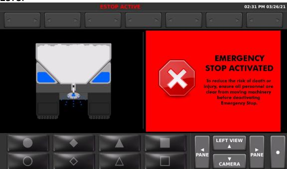
The SSC6100 has an emergency stop feature that is activated by pressing the red ESTOP pushbutton located near the Operator Interface control. When ESTOP is activated the screen shows the red Emergency Stop Activated message and a buzzer sounds. In addition, all outputs are immediately shut off, the system enters Standby mode, and if the system is configured with a Low Oil PTO or diverter valve, these will be shut off as well.
