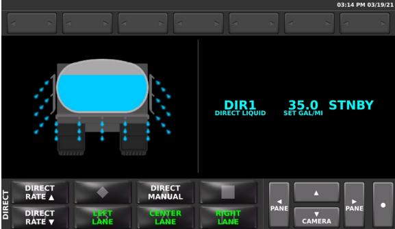
Direct Liquid Application mode is used to apply liquid deicing material directly to the pavement.
