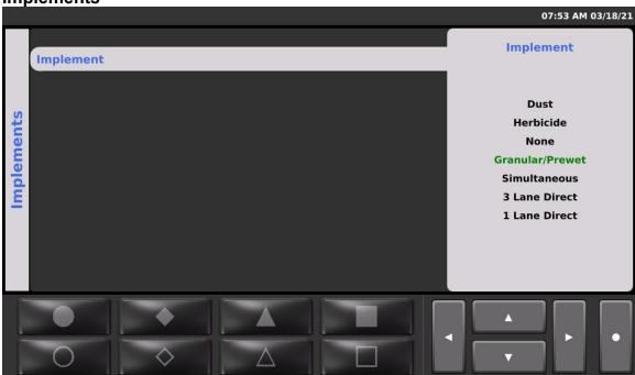
The SSC6100 system can optionally be configured to operate multiple types of equipment allowing the vehicle to be tailored for spreading various materials or performing seasonal work. These configurations are called Implements.
