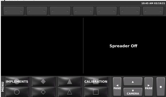
The 6100 system operates many aspects of the hydraulic system including joystick and spreader functions. For off-season use where the spreader controls are not required, a Spreader Power rocker switch can be used to remove the spreader functions from the operation screen and prevent outputs from being activated.
