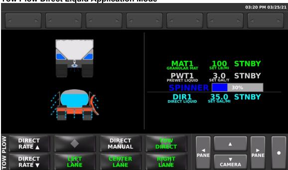
Direct Liquid Application Tow Plow mode allows the application of liquid material from an attached tow plow while spreading material from the truck. The liquid rate and lanes are separately controlled from the truck.
