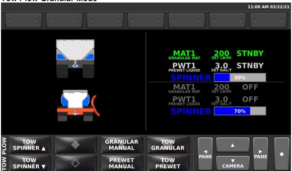
Granular Tow Plow mode allows the application of granular material from an attached tow plow while spreading material from the truck. The granular and prewet rates for the tow plow will be set to the same rates as the truck. See the section on Granular / Prewet Application Mode for information on adjusting these settings.
