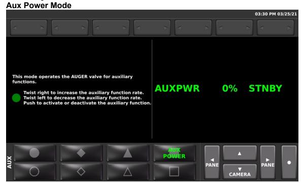
The Aux Power option allows the use of hydraulic flow from the Auger circuit to be used to power hydraulic tools and other functions. When enabled in Calibration, the AUX Soft Switch Pane provides the ability to enable this function.
