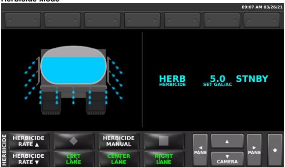
Herbicide mode allows for applying herbicides based on an area calculation. Multiple lanes are optionally supported.
