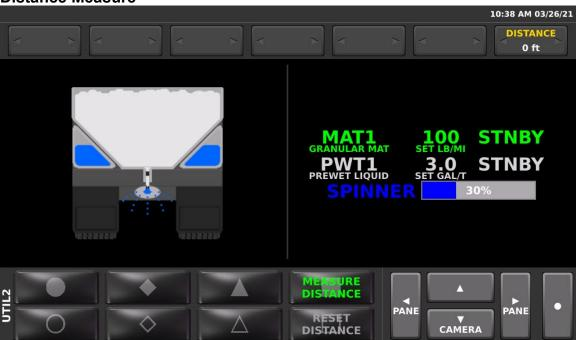
When enabled, the SSC6100 can perform a distance measuring function by using the ground speed signal from the vehicle. The distance traveled by the vehicle is shown with an option to reset the distance value and start a new measurement.
