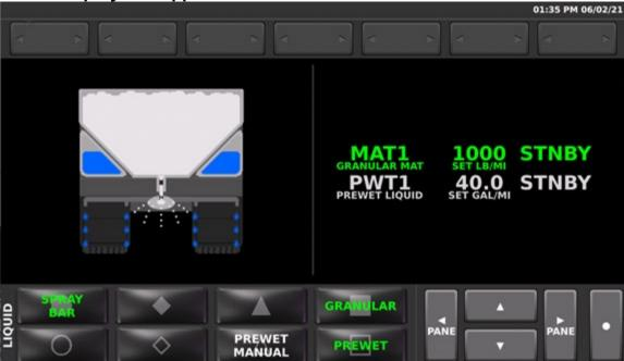
This mode applies granular / prewetted material with the option to apply prewet liquid directly through a spray bar.
