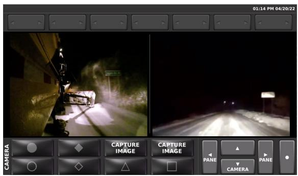
The SSC6100 can support up to three different video camera inputs and various display options on the screen. A single live video from one of the cameras can be selected to show on the left screen. Also, two live cameras can be selected to show on the left and right screens
