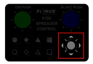
The touch screen navigation controls area and Nav Stick joystick provides a way to change between views on the screen, select panes of Soft Switches, and make adjustments to settings. The up, down, left, right, and select functions can be done using Nav Stick on the operator interface or also with the touchscreen on the display.
