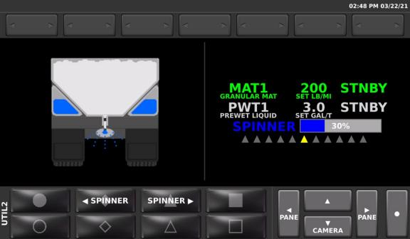
Directional spinner is an option for granular systems that adds the ability to position a spinner that can be used to aim the granular material to the left or right. It uses a position sensor to show the relative position of the spinner on screen as a yellow triangle under the spinner speed.
