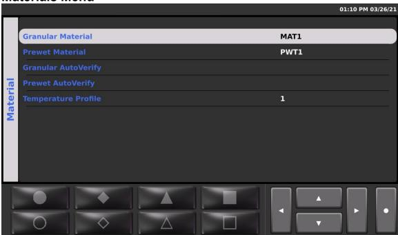
The Material Selection Menu allows you to choose between different materials for each of the spreading modes. The list of available materials is configured and calibrated for each mode in the Calibration settings.
