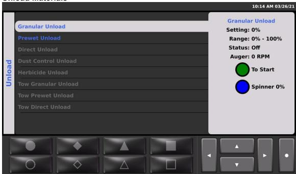
The SSC6100 provides a means of unloading leftover material by manually running the associated hydraulic function at a set speed. If enabled, the Unload menu is accessed from the MENU Soft Switch pane by pressing the Unload button.
