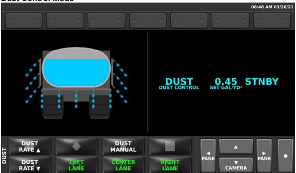
Dust control allows for applying dust control liquids based on an area calculation. Multiple lanes are optionally supported.
