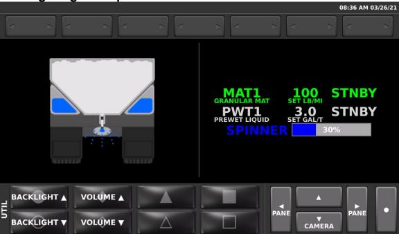
The intensity of the LCD backlighting and volume of the speaker can be adjusted on the UTIL Soft Switch pane. As the speaker volume is adjusted, the speaker sounds a tone to show how loud or soft the setting is.
