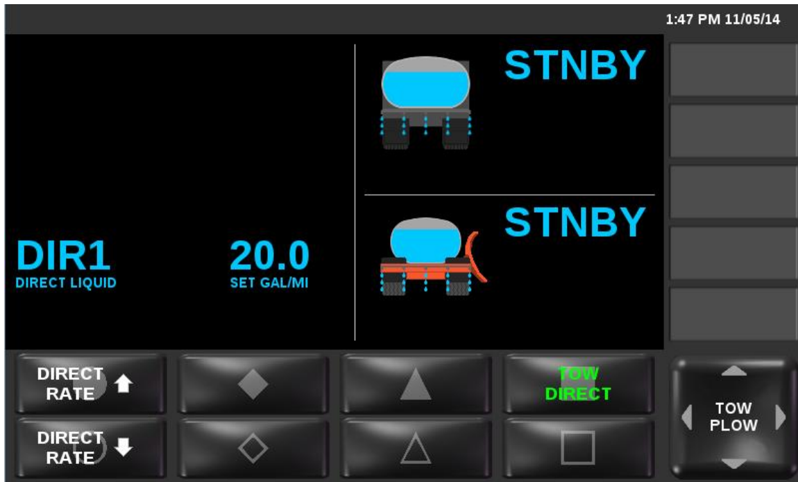
Figure 34: Truck Direct with Tow Plow Direct Application Mode
