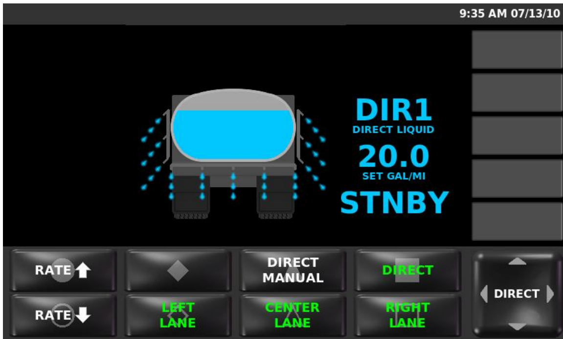
Figure 23: Direct Liquid Multi-Lane Application Mode
