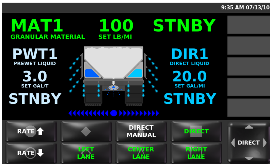
Figure 26: Simultaneous Granular / Prewet / Direct Application Mode
