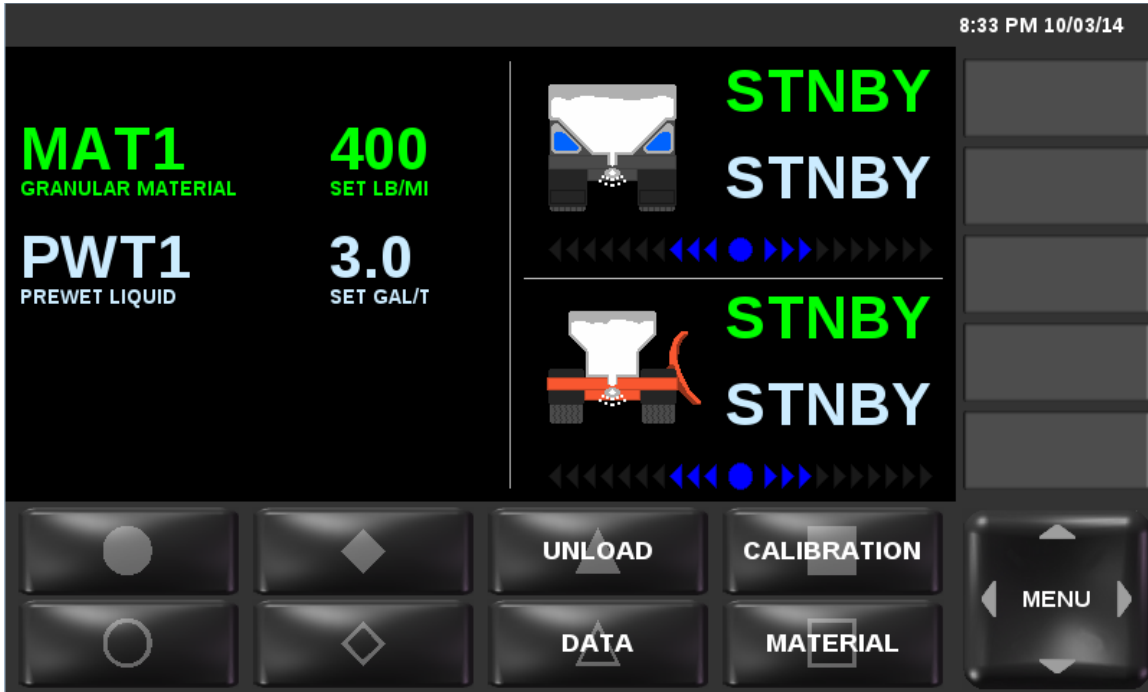
Figure 33: Truck and Tow Plow Granular and Prewet Application Mode
