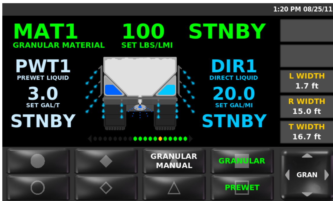
Figure 30: Directional Spinner Application Mode
