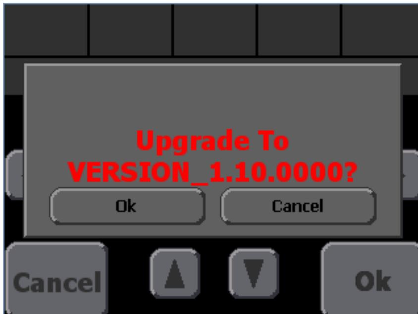
**Figure 15: Upgrade Firmware File Confirmation**
