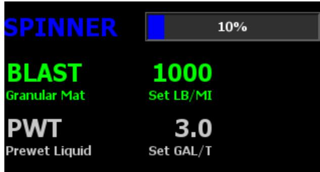
Figure 9: Granular / Prewet Application Mode in Blast
