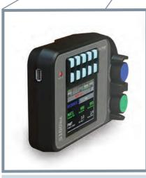
Built-in USB port for data retrieval and firmware upgrades.
