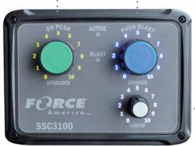
Color LEDs around the dials illuminate the numbers as rates are increased.
