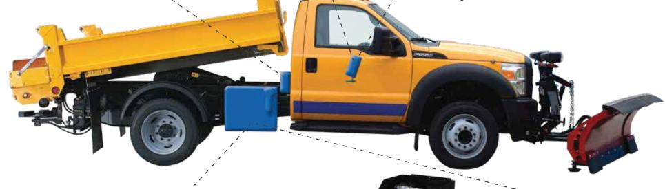
VT12: 12.3 gallon tank with powder coated steel valve enclosure offers protection and easy serviceability
